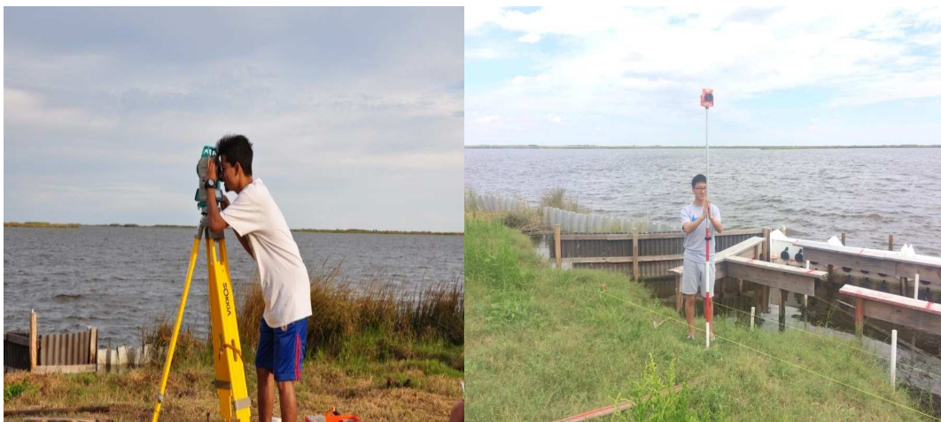
Figure 17: Surveying Technique for SET Measurements
